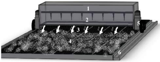
Fig. 3. The actuator mounted on the PV panel 1) HV electrode; 2) Ground electrode; 3) Exit of the ionic wind; 4) Dust; 5) Driven wheel; 6) Guide rail.
